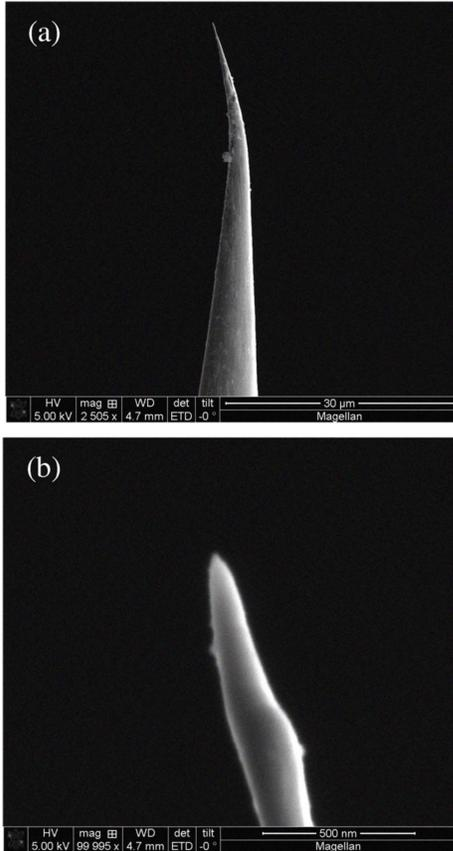
Fig. 2. SEM micrograph of tungsten probe fabricated using the TEE approach: (a) ~2.5× magnification, and (b) 100,000× magnification.
