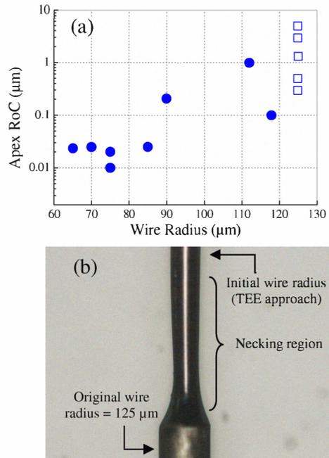
Fig. 1. (a) Plot of tungsten probe apex RoC versus initial wire radius utilizing the single-step (hollow squares), and two-step (solid circles) DC dynamic electrochemical etching procedures. (b) Microscope image of the tungsten wire showing the necking region, original and initial tungsten wire radius fabricated using the TEE approach.
